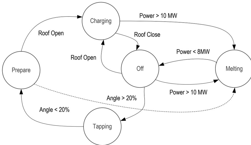
**Figure 3 - Simplified Finite State Diagram for EAF**
