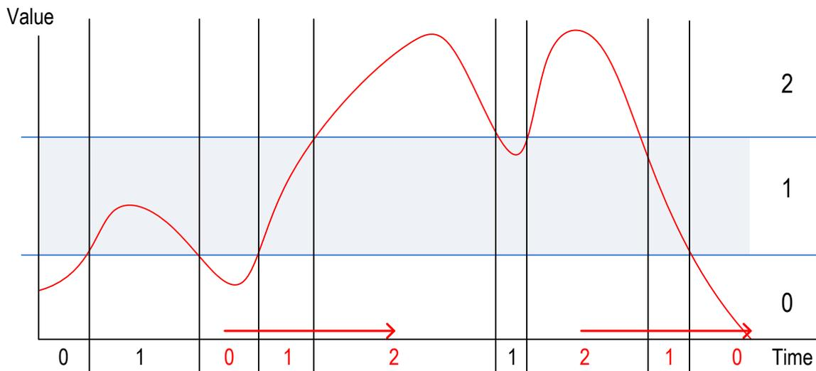
**Figure 3 - Calculation of events on an analog variable**
