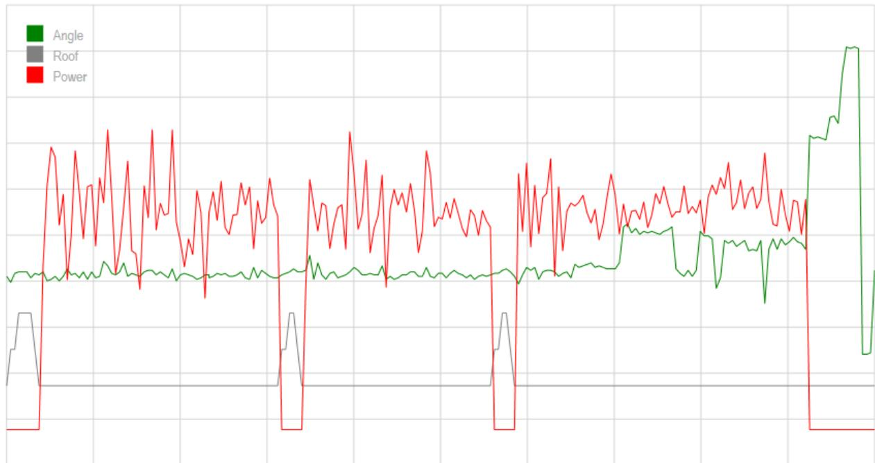
**Figure 1 - Actual EAF Heat fingerprint**
