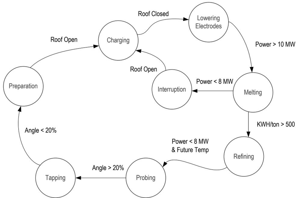
**Figure 2 - Finite State Diagram for EAF process**
