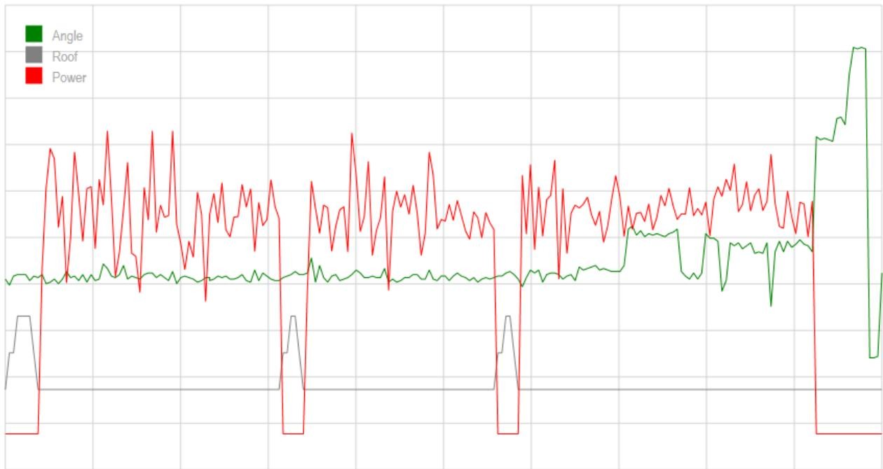
**Figure 1 - Actual EAF Heat fingerprint**
