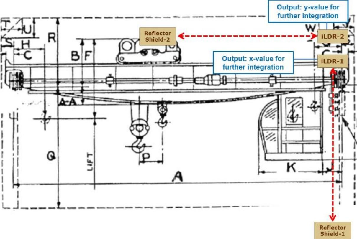
Illustration: Crane with equipment in installation positions + connections.
