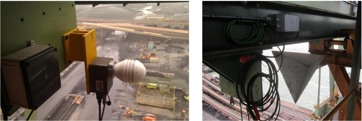
Illustration & Images: This iLDR™ cabin positioning solution with the iLDR™ sensor (left, exposed to sea spray, rain and fog, and in full operation) and the reflector shield (right) which does not need to be powered
