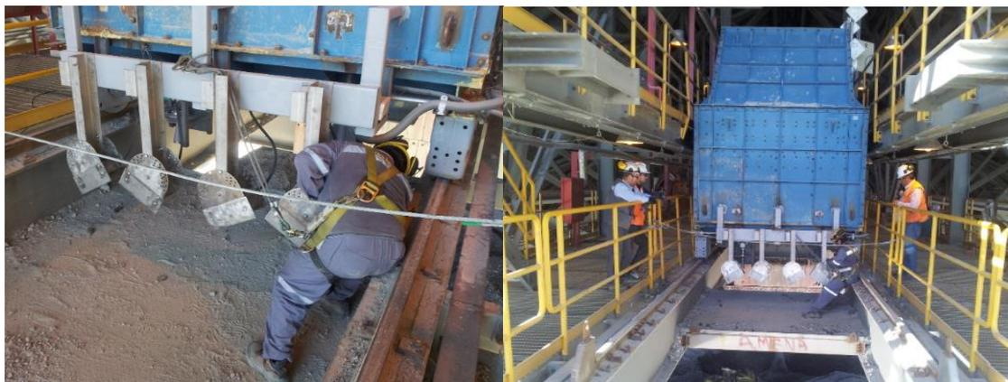
Photographs: iStockpile™ installation example with 4 iStockpile™ iDRR™ sensors installed
