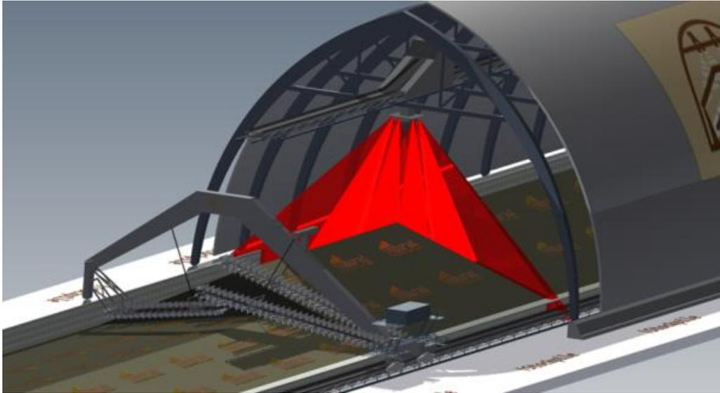
Illustration: Typical iStockpile™ installation environments with radar beams in red
