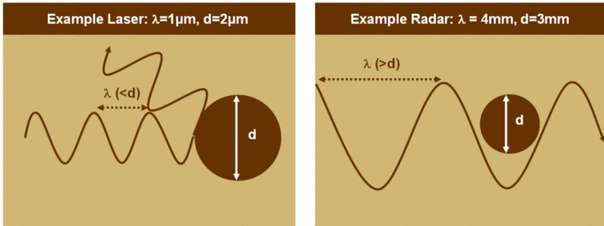
Illustration: Performance of Laser (left) and Radar electromagnetic waves in heavy-dust environments
