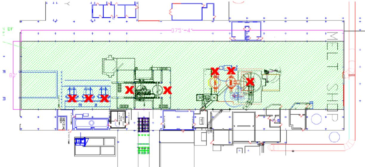
Illustration: View from above Red x represent areas of required alarm if crane moves into/above these
