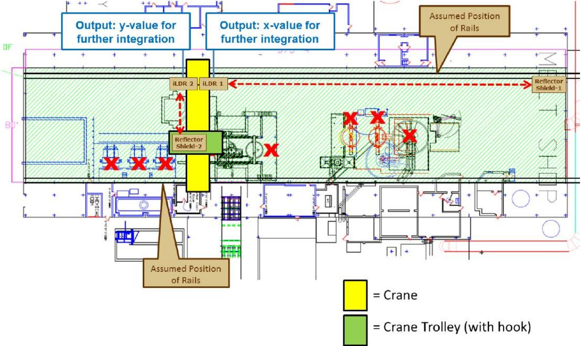
Illustration: View from above, showing all equipment in approximate installation positions + connections.
